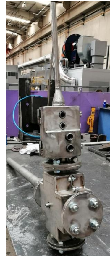
O 2 injection system
